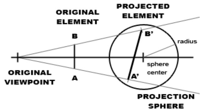
Fig. 14 – example of the projection of a triangle side
